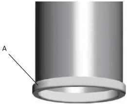
4. Fit the gasket (A) onto the edge of the flue pipe.
