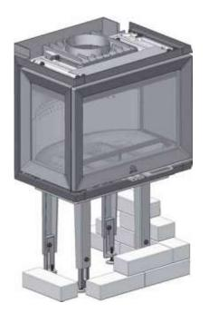
1. The bricks are laid so that they fit under the insert frame.
