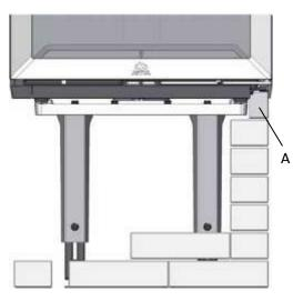
2. The last bricks (A) are cut to fit between the leg base and the frame. NB: Remember to leave openings in the brickwork for convection air (Fig. 1 e and f).
